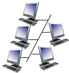
shared wire (e.g., cabled Ethernet)
