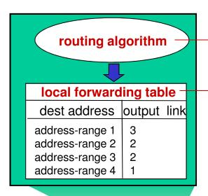
routing algorithm determines end-end-path through network
