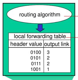
routing algorithm determines end-end-path through network
