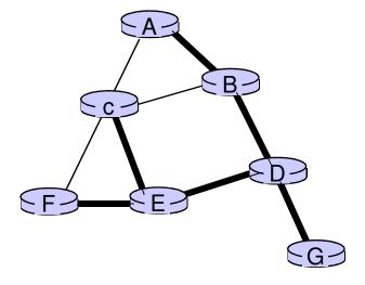
(b) constructed spanning tree
