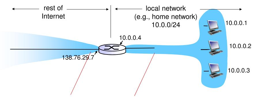
all datagrams leaving local network have same single source NAT IP address: 138.76.29.7, different source port numbers datagrams with source or destination in this network have 10.0.0/24 address for source, destination (as usual)
