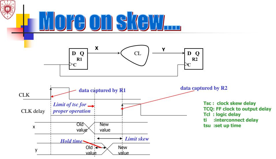
If the data changes fast at y and skew was large as shown, y can change and the edge of clock will capture the new data. In this case there is a race situation and there is a limit on the clock skew to capture the old data.
