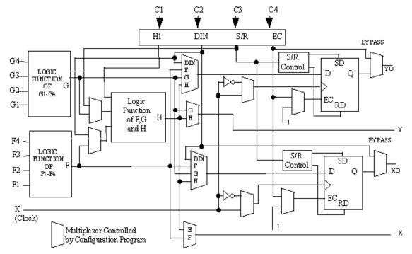
Block Diagram of XC4000 Families Configuration Logic Block (CLB)
