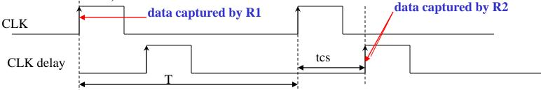
Skew extends the period, so the actual clock period can be "the reduced original Clock period". To take care of this:  $t_{actual} = t_{CQ(max)} + t_{CL}(max) + t_i(max) + t_{su}(max) - t_{cs}(hin)$
