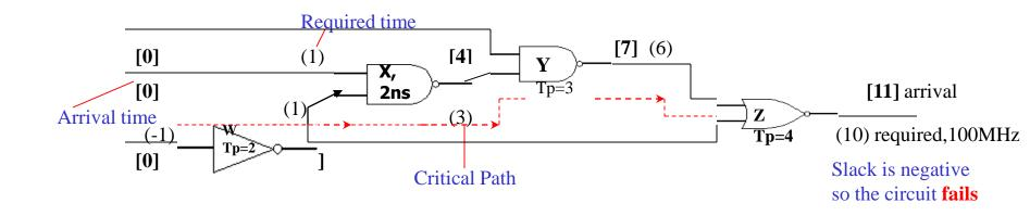
**Solution:** Signal C should arrive 1 ns earlier or reduce delays in the critical path ( i.e. re-design building block or circuit ).
