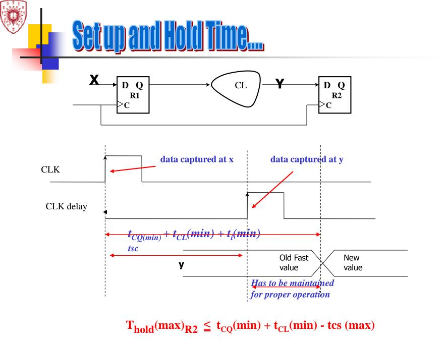
$t_{CL} = t_{logic} + t_{interconnect}$
