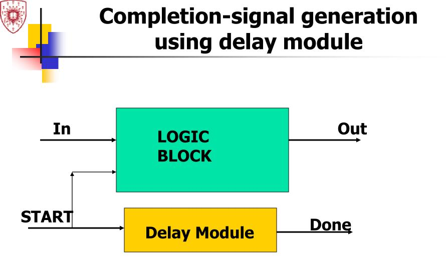
•This mechanism helps to establish the precise duration of a computation in a data-path fashion(taking care of physical constraints).
