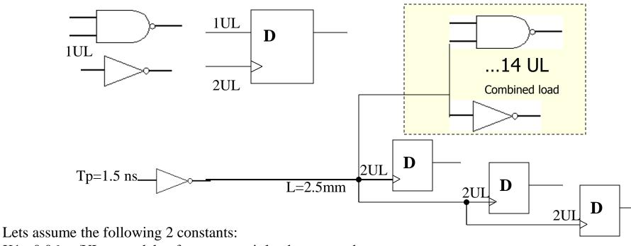
K1=0.06 ns/UL delay factor per unit load connected
