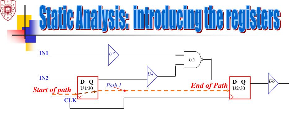
**Path 1** goes from CLK to Q on Register U1 through U4 buffer and U5 NAND gate to the D input of U2. Path analysis adds up the delay along this path and compares the total with the clock arrival time at U2. Example: Assuming:
