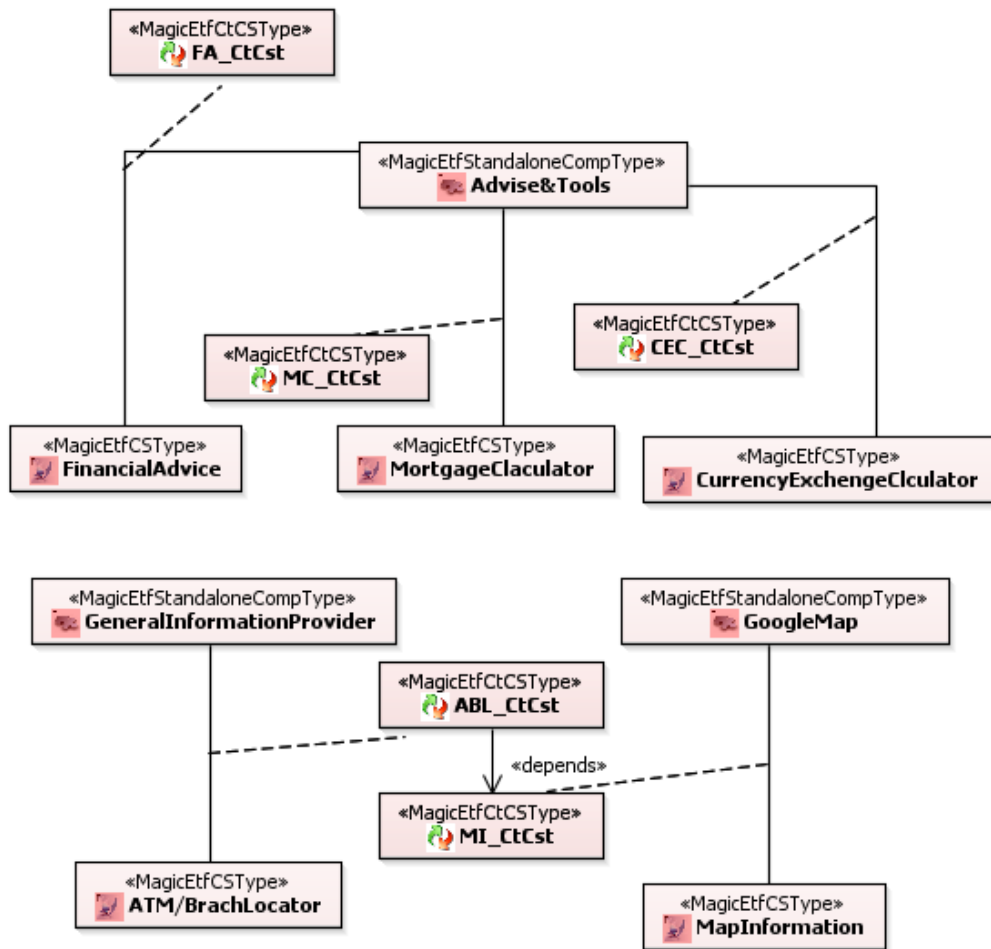
Figure 7-8 ETF model for the general inquiries part of an online banking software bundle
