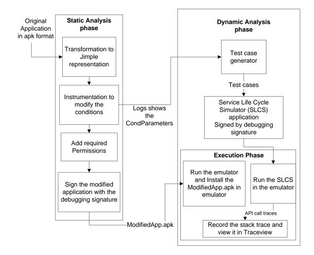
Figure 6.1 HyDroid Approach for extracting API call traces from Android app services in the presence of obfuscation
