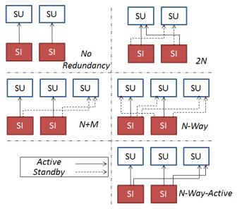
Figure 1. Redundancy models defined in the AMF specification
